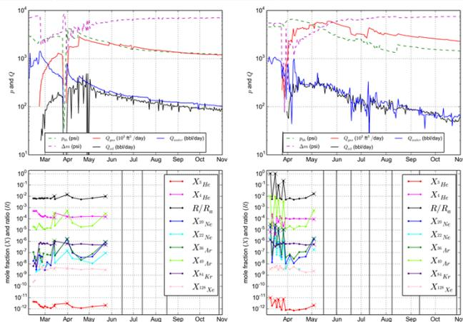
Production (top) and Noble gas compositional (bottom) data for two shale gas wells
