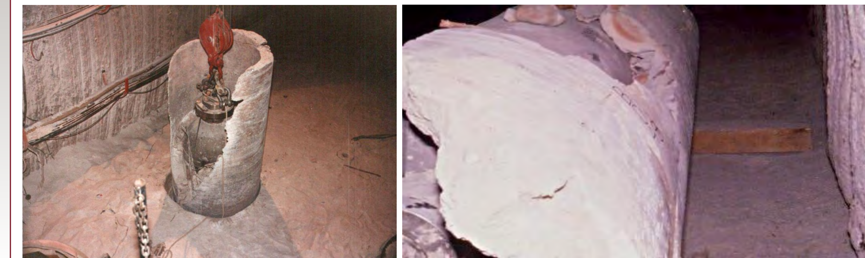
Figure 7: Images of heaters during overcoring and removal at WIPP Room B (Kuhlman et al. 2017).
