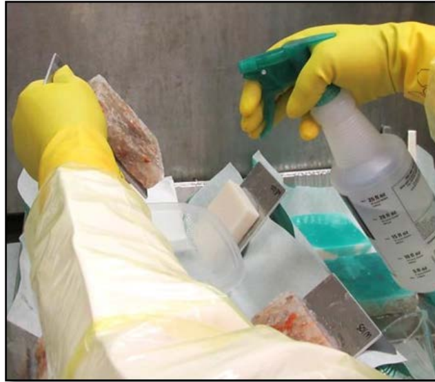
Figure 3. Laboratory test at INL to determine quantities of brine required to clean actinides from salt (INL, 2014)
