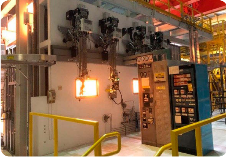
Workers recently installed manipulator equipment at a full-scale mock-up of areas of the Hanford Site's Waste Encapsulation and Storage Facility. (Photo: DOE)
