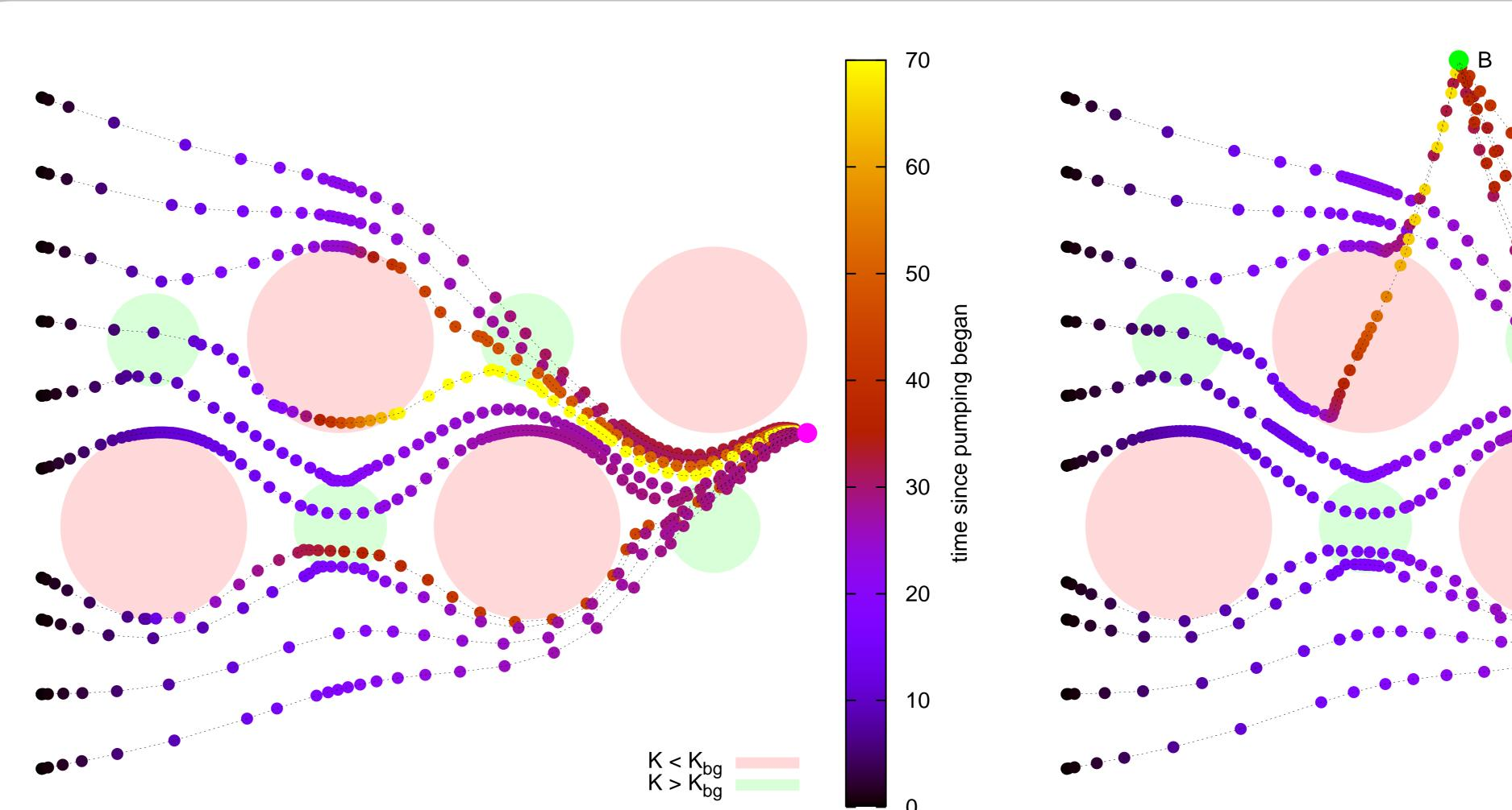
These plots show traces of particles released along the left edge of each figure. On the left, a single pumping well operates at a constant rate until the particle are captured, while on the right well A shuts down and well B starts up at t = 30. Dot colors indicate time since pumping began.  $K_{\text{bg}}$  is the background hydraulic conductivity (white areas in the figures).
